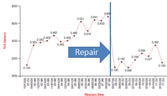
In this case, machine vibration increased gradually. Two tests per year is sufficient to detect the problem before failure occurs. (Fig. 6-2)
